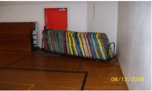
Photograph 2 – Taken at North Fond du Lac on December 8, 2009, showing a rack of folding chairs blocking an exit.
