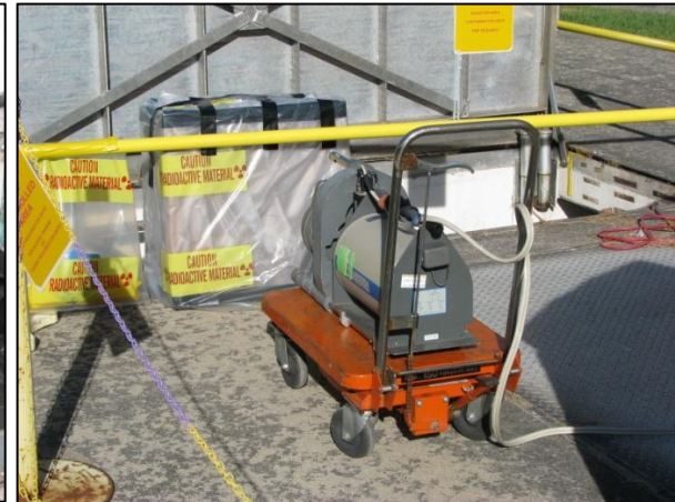
ISOCS Survey of Removed HEPA Filter
