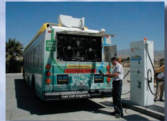
Fueling the XCELLSIS fuel cell bus with compressed hydrogen. Photograph courtesy of Bob Barnitt, eTIAx LLC. (Department of Energy/National Renewable Energy Laboratory).
