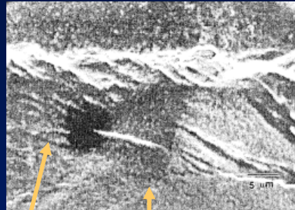
Hour and Stubbins (1989) – Alloy 800H, fatigue crack growth
