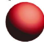
Dia. 0,5mm Uranium Dioxide Fuel Kernel
