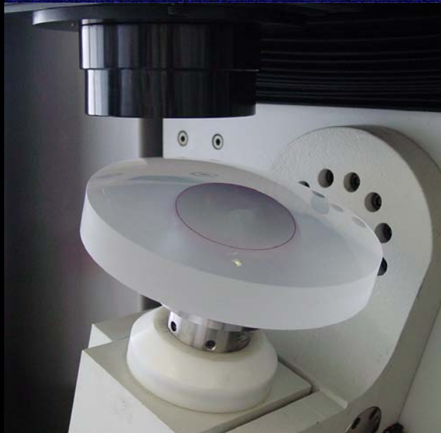
Large aperture lens mounted in QED's SSI.
