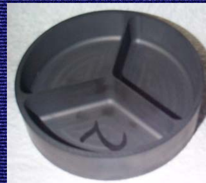
CoorsTek lightweight SiC mirror 20 kg/m 2
