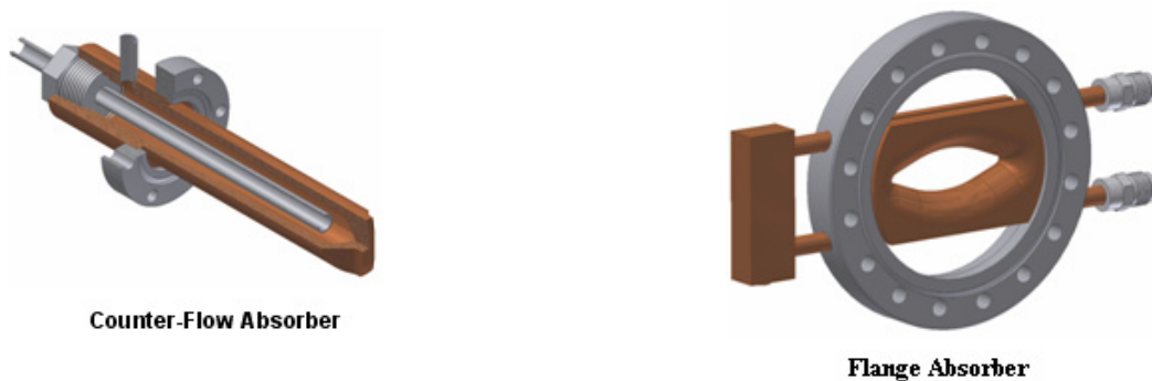
Figure 7.7.9 Counter-flow and flange absorbers for the storage ring vacuum chambers.
