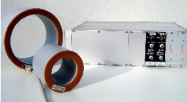
Figure 4.9.4 Bergoz NPCT (New Parametric Current Transformer).
