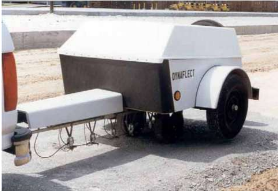
Figure 8. Dynaflect Deflection Trailer
