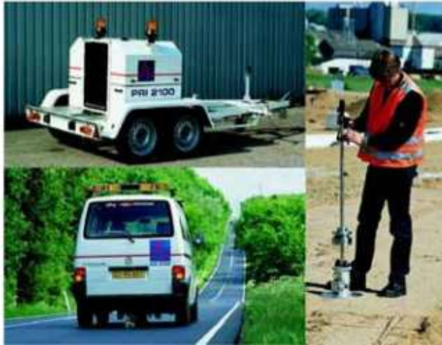
Figure 12. Carl Bro FWD/HWD and LWD Trailer, Van-Integrated or Portable
