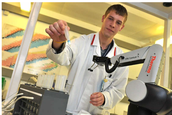
Figure 3: Robot arm system used in NML for automated processing of highly radioactive spent fuel samples.
