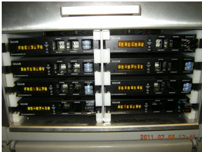
Figure 4: The NGAM (Next Generation ADAM) module is a 8 channel SCA data acquisition module. It is backward compatible with all VIFM system detectors. Data is stored redundantly on two discrete drives. It is a TCP-IP compliant device that connects to collect computer via an Ethernet (internet/intranet) connection. The NGAM also features an embedded web-browser application that allows data archive and system diagnostics via a PC (i.e. without need of connection to a collect computer or additional software).
