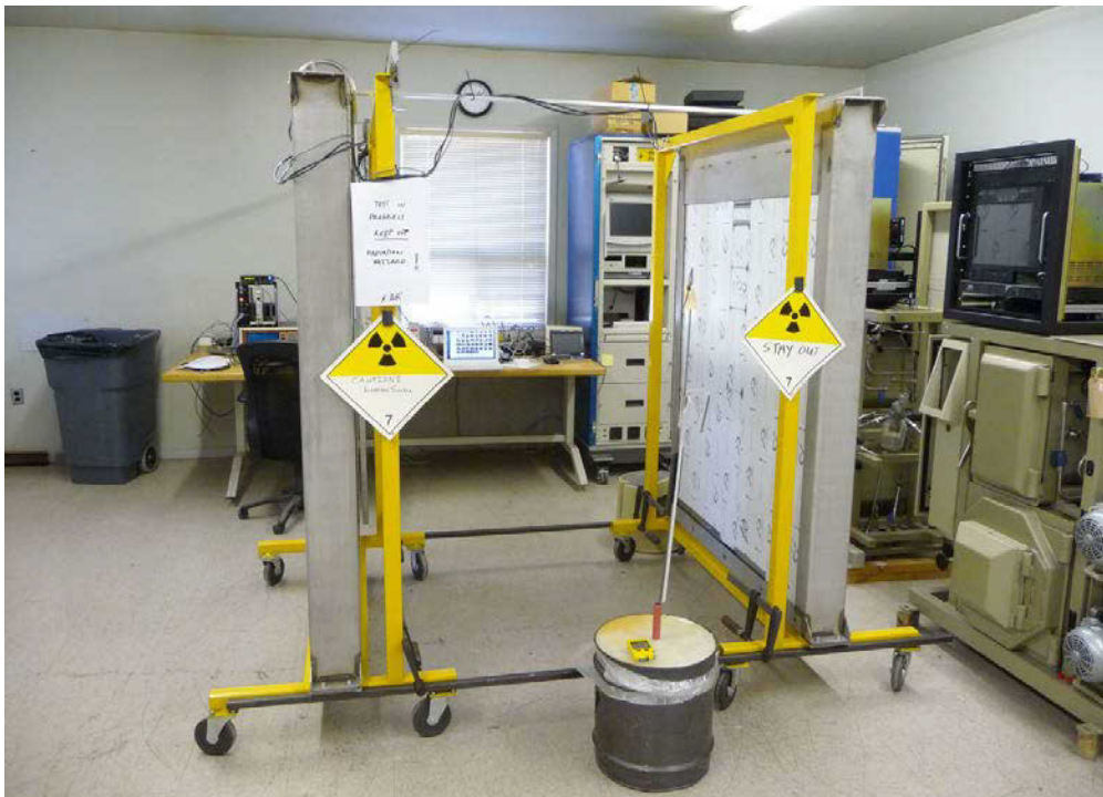
Figure 2: Testing of AMGB Prototype during Factory Acceptance Test.
