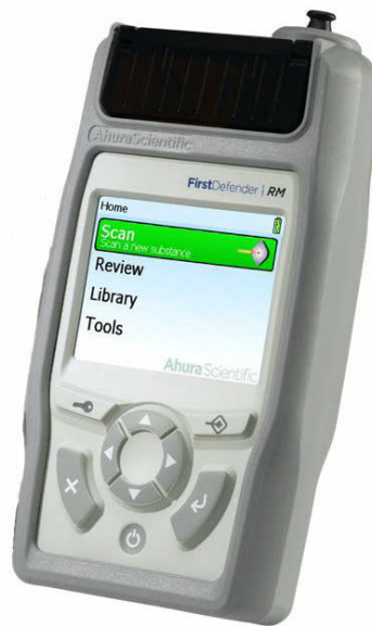
Figure 1: Handheld Raman System (HHRM) based on the commercially-available FirstDefender RM . The system uses Raman Spectroscopy to matched target material with library scans in its memory. It can store over 7,000 material scans in its library. The system as supplied can identify a wide range of light-coloured and non-fluorescent compounds.
