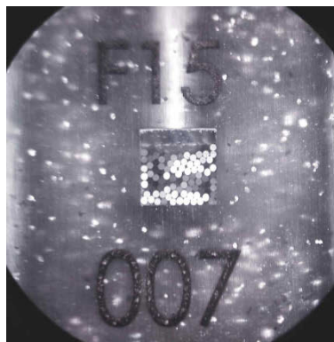
Figure 3: Modified iCOBRA seal with Reflective Particle Tags (RPT) and a verification image.
