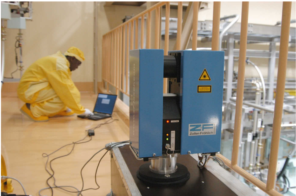
Figure 3: 3DLR laser scanner used by SG inspector.
