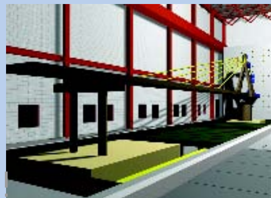
As a part of NEES, the Structural Engineering and Earthquake Simulation Laboratory at the University at Buffalo, State University of New York, is upgraded with dual shake tables to enable researchers to investigate the behavior of large structural systems and components when subjected to complex seismic excitations at a scale and complexity not previously possible. The laboratory has a modular and highly flexible framework that allows multiple configurations of full-scale and component tests combined simultaneously with real-time numerical simulations. This illustration is from an animation that depicts a bridge experiment in the new facility. Illustration courtesy of University at Buffalo, SUNY, Structural Engineering and Earthquake Simulation Laboratory
