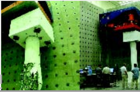
The NEES facility at the University of Illinois at Urbana-Champaign has three large capacity load and boundary condition boxes (LBCB). The photo shows one LBCB mounted to the reaction wall and a bridge pier to test the bridge pier response during an earthquake. The bridge pier is part of a large model of the Santa Monica Freeway (I-10) that suffered extensive damage in the 1994 Northridge, California earthquake. A computer model representing the rest of the freeway was running in parallel during the test. The successful replication of the failure of the freeway during the test, as evidenced by the damage to the bridge pier in the photo, will enable engineers to improve the seismic design of future structures. Photo courtesy of University of Illinois at Urbana-Champaign
