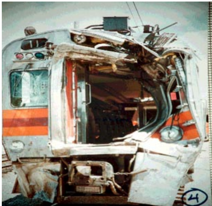
Figure 4. West (damaged) end of NICTD car 11
