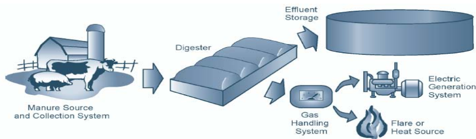
Figure VII-7 Biogas Recovery Systems
