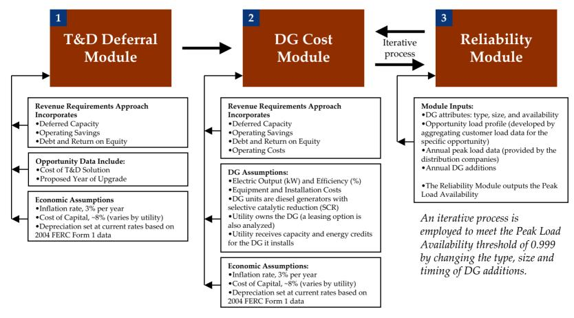
On an annual basis the cost of the DG solution is compared to the deferral savings. When the annual cost of the DG solution is greater than the annual savings of the T&D deferral, the deferral period ends.
