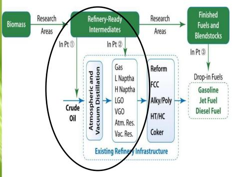
1 Jones, S., Valkenburg, C., Walton, C., Elliott, D., Holladay, J., Stevens, D., "Production of Gasoline and Diesel from Biomass via Fast Pyrolysis, Hydrotreating and Hydrocracking", Feb 2009 Biomass is converted to a bio-oil that can be co-processed with conventional crude
