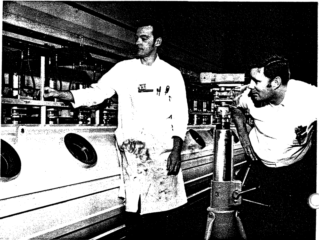
FIGURE III.2.g.1 Checking strong-back alignment.
