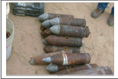
Holes are Drilled in Projectiles as Required by the Demil Manual
