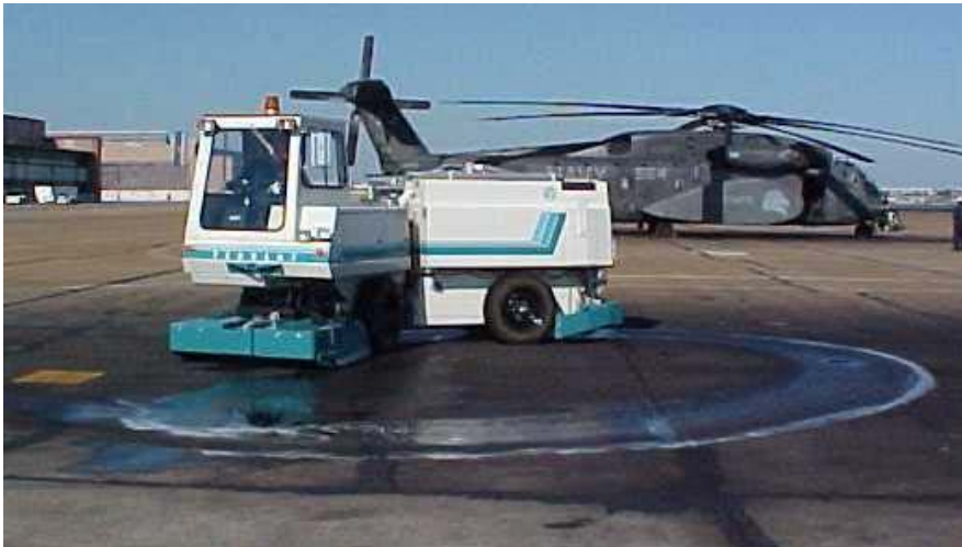
Cleaning oil stains on helicopter fueling area
