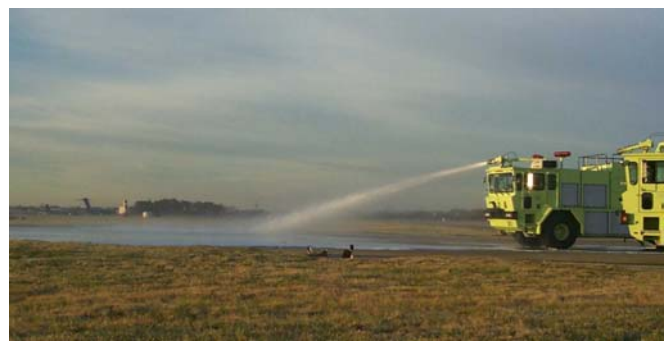
Crash truck discharging fire fighting foam onto washrack
