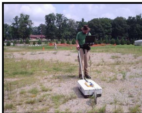
Ground Penetrating Radar (GPR) survey used to identify geophysical anomalies at OU 4.
