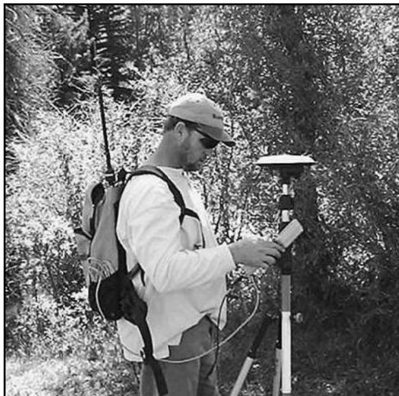
Identifying the location of federal interest lands assists in streamlining development of renewable energy and other purposes while preserving locations of boundaries established in the 1800s. The BLM employs the latest in survey-grade GPS technology in identifying the positions of original survey corner evidence.
