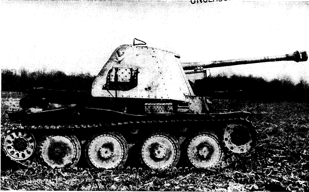
Figure 82.—7.5 cm Pak 40 on Pz. Kpfw. 38 (t) Chassis.
