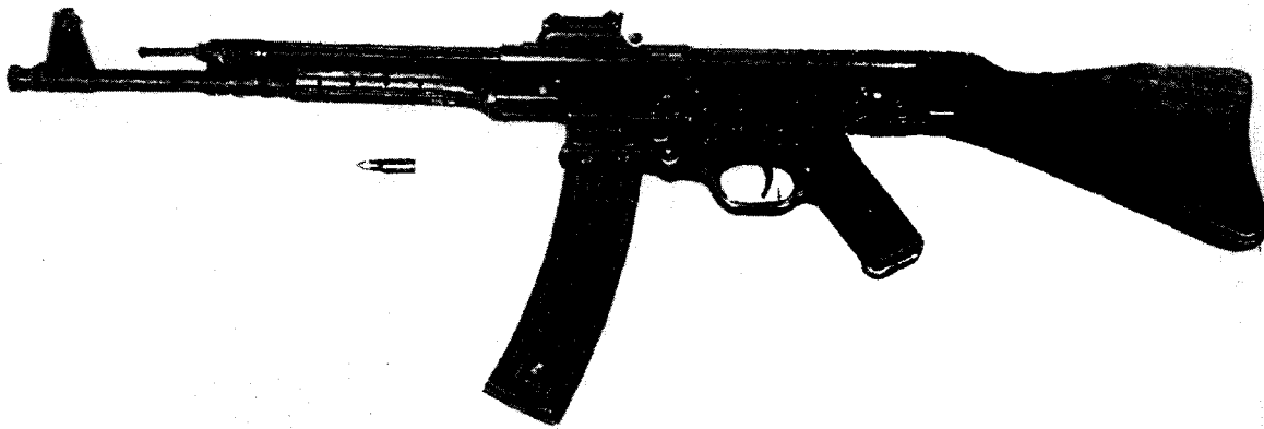
Figure 7.—M.P. 43/1, caliber 7.92 mm, showing magazine in place for firing.
