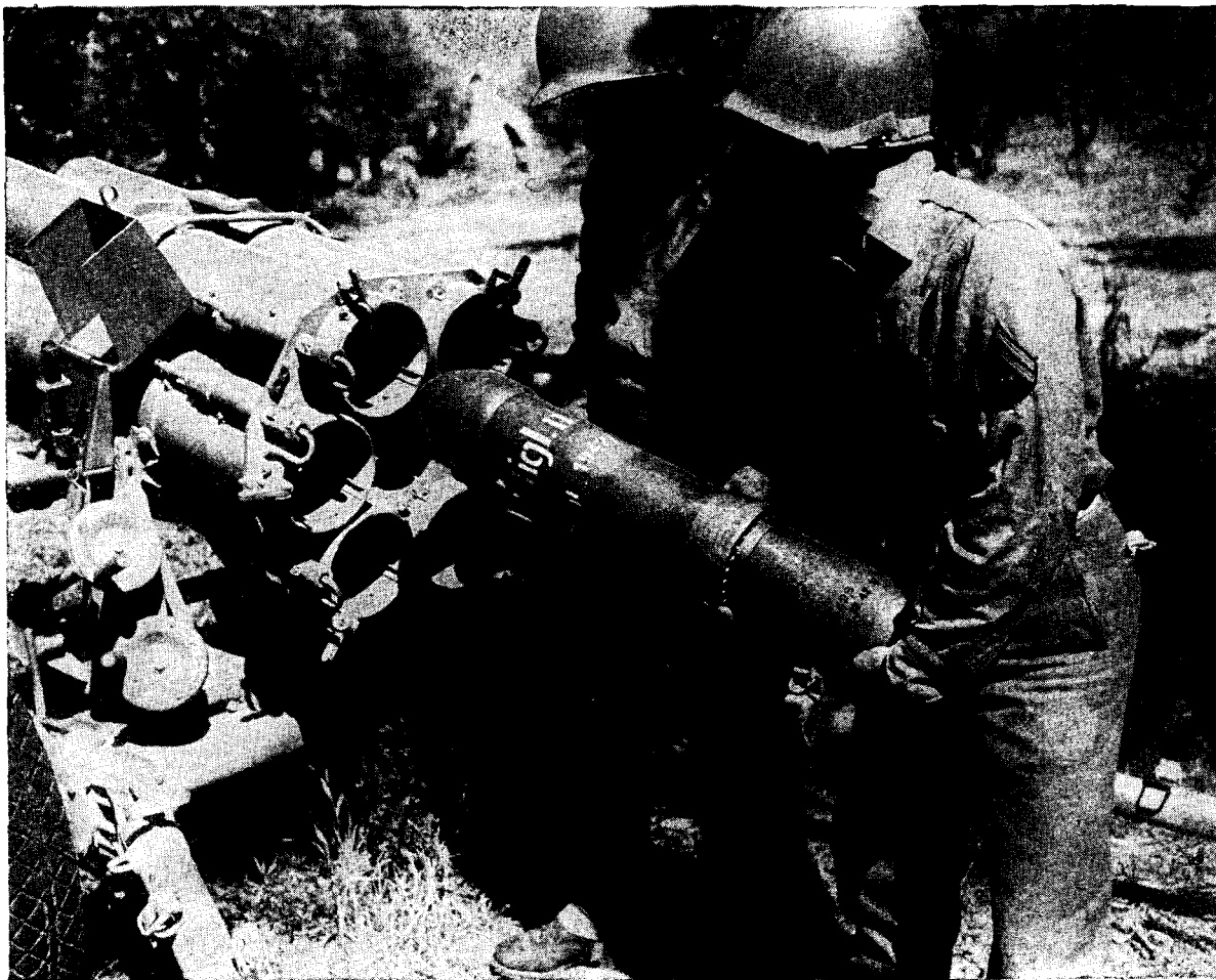
Figure 127.—15 cm Nebelwerfer 41 being loaded.
