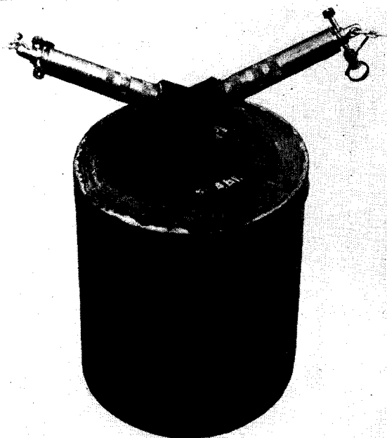
Figure 72.—S-Mine with Y Adapter and Z.Z. 35 Igniter.
