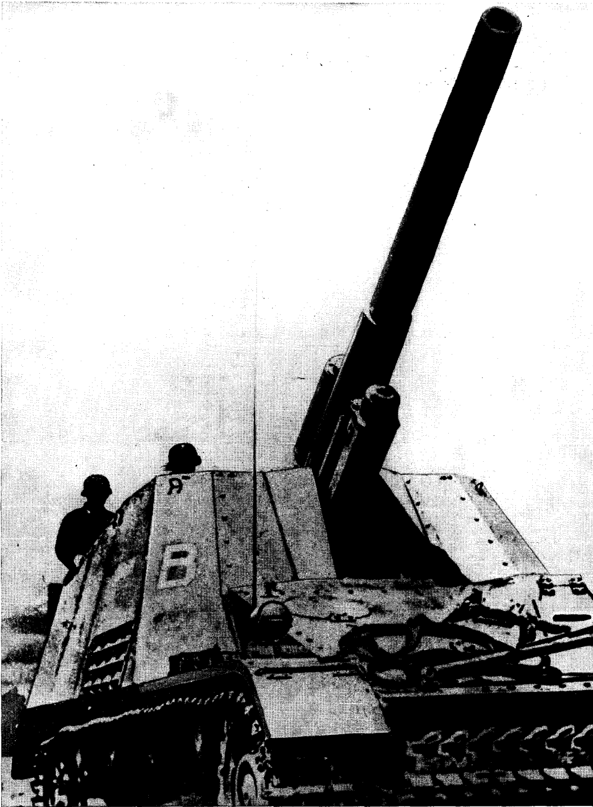
Figure 91.—15 cm. s.F.H. 18 on hybrid Pz. Kpfw. III/IV Chassis (Hummel).
