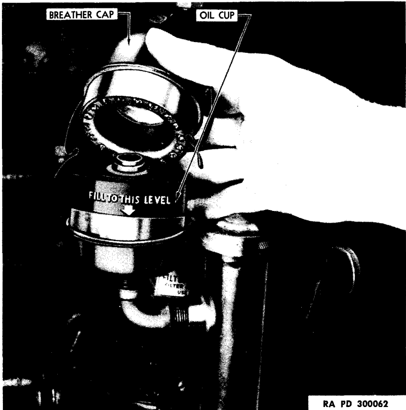
Figure 29—Crankcase Ventilator and Air Cleaner
