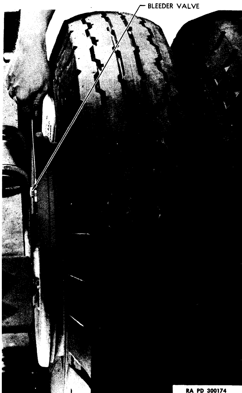
Figure 84—Bleeding Rear Brake
