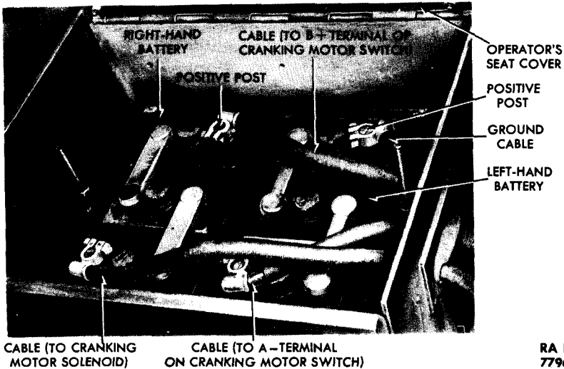
Figure 97 – Batteries Installed
