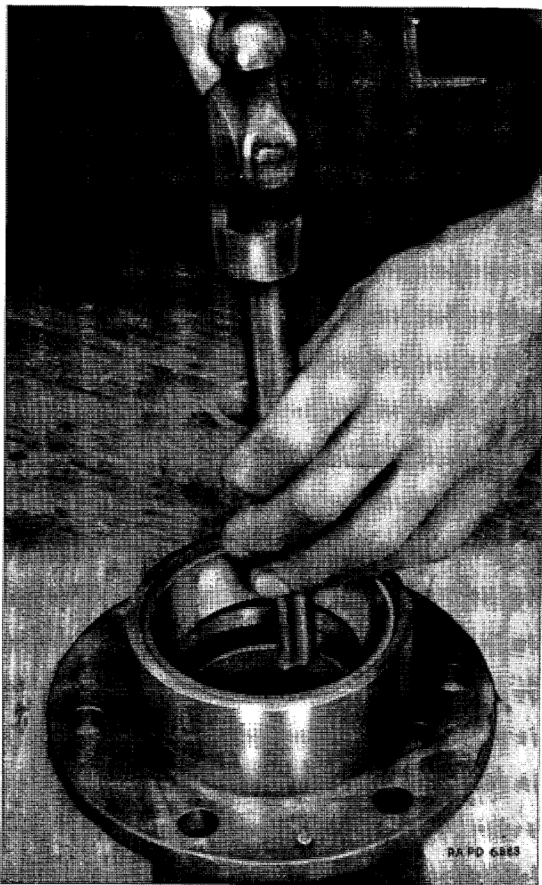
FIGURE 24.—Front axle drive pinion bearing cup removal.
