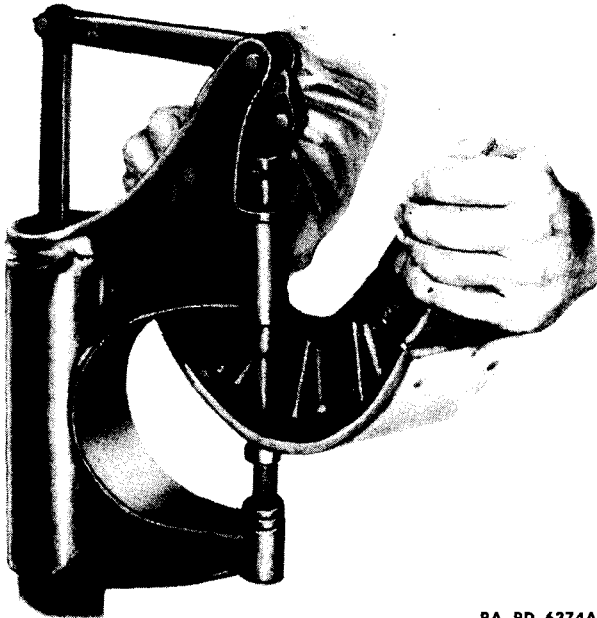
Figure 87—Riveting Brake Lining
