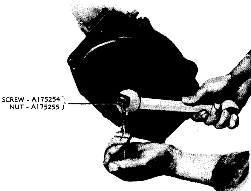
Figure 161—Steering Gear Lever Shaft End Play Adjustment
