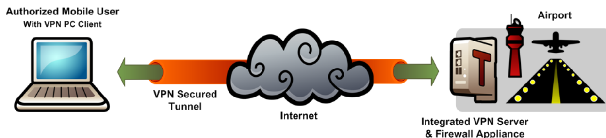
Figure 1. Secure access to critical systems for remote support personnel
