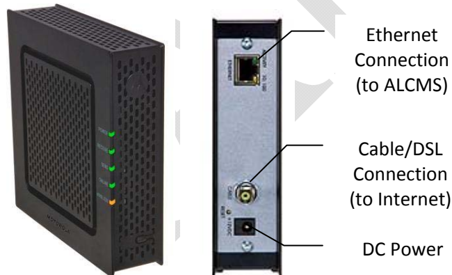
Figure 4. Typical external gateway appliance (image courtesy of Motorola Inc.)
