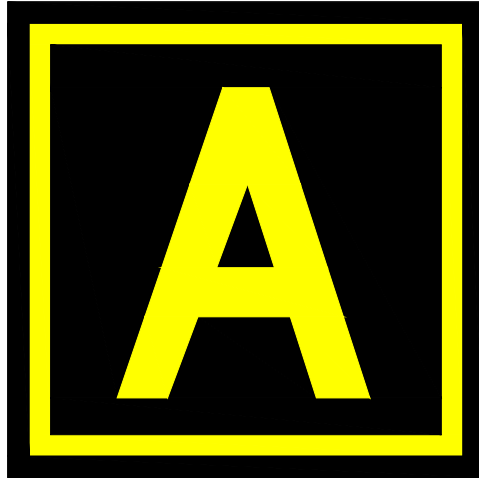
(a) Taxiway Location Sign
