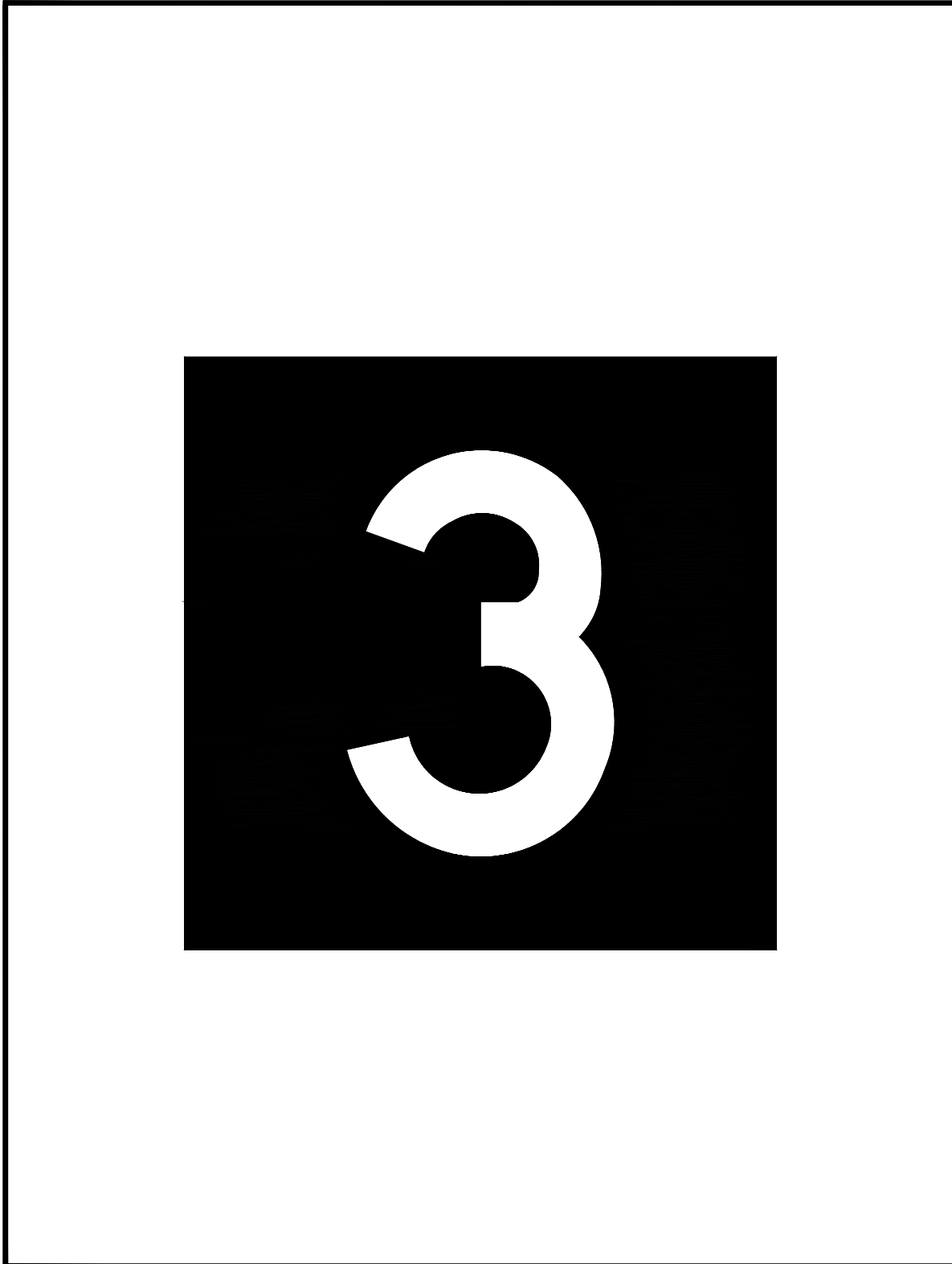
Figure 15. Runway Distance Remaining Sign.
