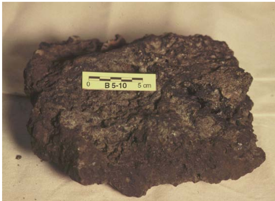
Figure 1-3. Hand sample of Site B slag. This sample is dominated by glass and is apparently a cooling surface of the slag. (Photograph courtesy of CNWRA).
