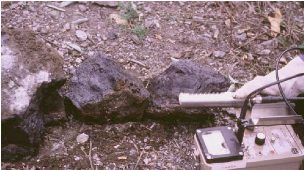
Figure 3-1. Weathered Slags from Sites A and B. Top photograph is of a Site A sample after it was split into two pieces. The contrast between a weathered and unweathered surface can be seen in the block in the foreground. The outer weathered surface is visible on the right edge of the block and it is a reddish brown material several mm thick. The unweathered interior is visible on the left and the alternating light and dark layers show up well. The lower photograph is of Site B sample B-5.5 after being split in the field. The outer weathered surface is visible on the top of the block on the left. It is a light tan color and is several mm thick. The unweathered interior is very dark gray in color.
