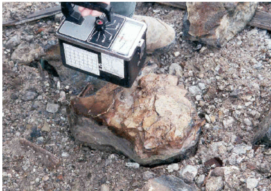
Figure 1-6. Close up of slag found at the ground surface at Site C. The interior is medium gray in color. The outer rusty brown colored surface is indicative of the rapid weathering of these blocks when exposed to the atmosphere.
