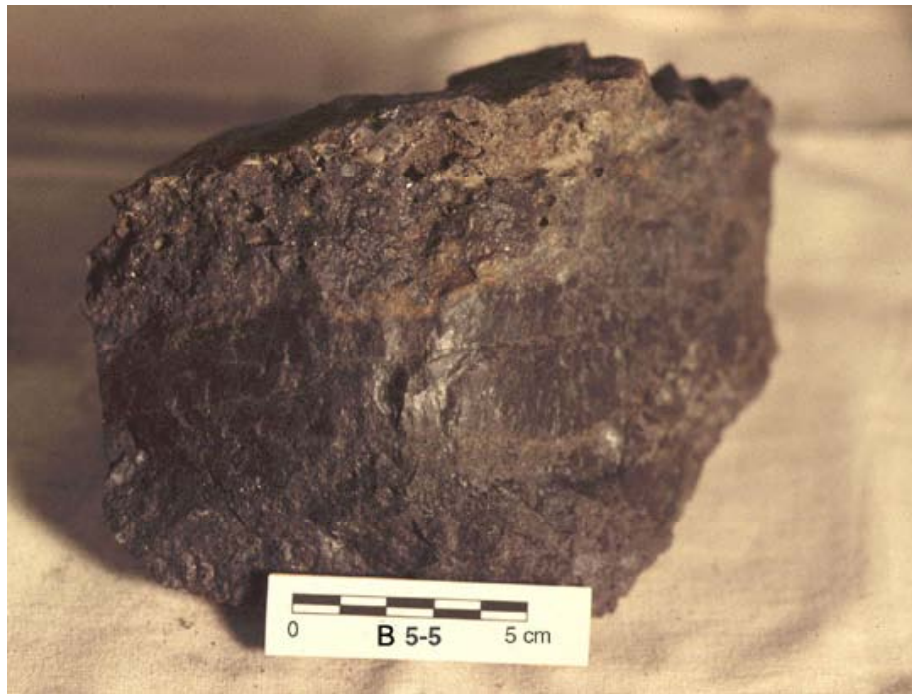
Figure 1-3. Hand sample of Site B slag. This sample is dominated by glass and is apparently a cooling surface of the slag. (Photograph courtesy of CNWRA).
