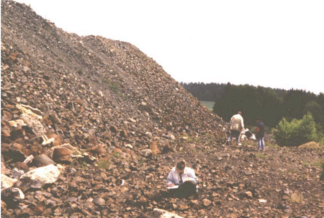
Figure 3-22. Pribram slag pile, Czech Republic. Pribram mine was the site of Pb, Ag, mining and smelting. This is a 10 - 30 year old slag pile. The surface weathers within several years to a buff or white color.
