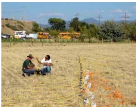
Dr. Kenneth H. Williams (LBNL) and graduate student Adrian Flores Orozco (University of Bonn) collecting surface spectral induced polarization data at the Rifle site to detect and delineate regions of naturally elevated subsurface microbial activity.
