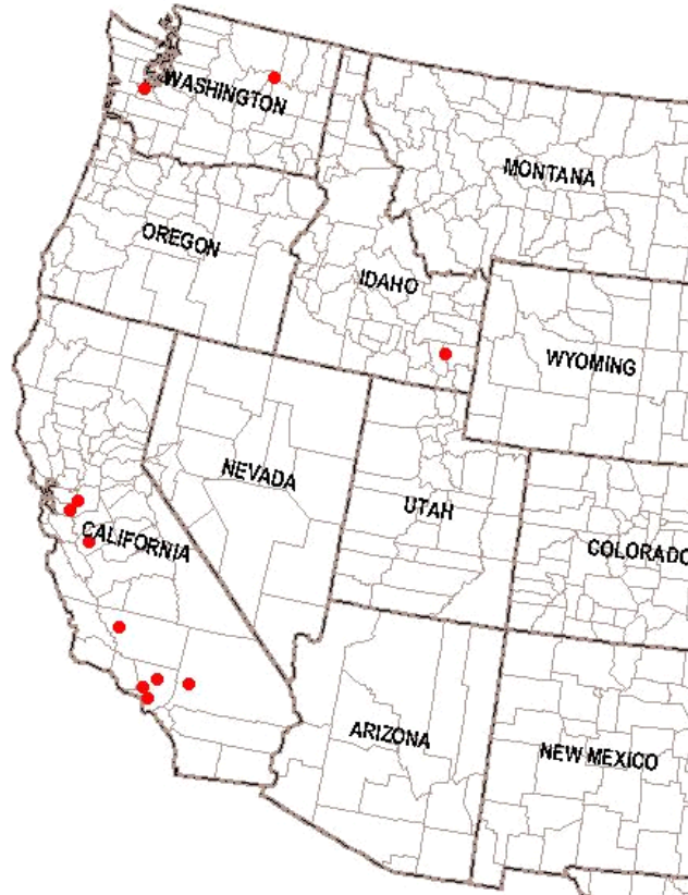
Figure 5-17. LA region - location of transformers at risk, GIC of 500 Amps or greater per phase.
