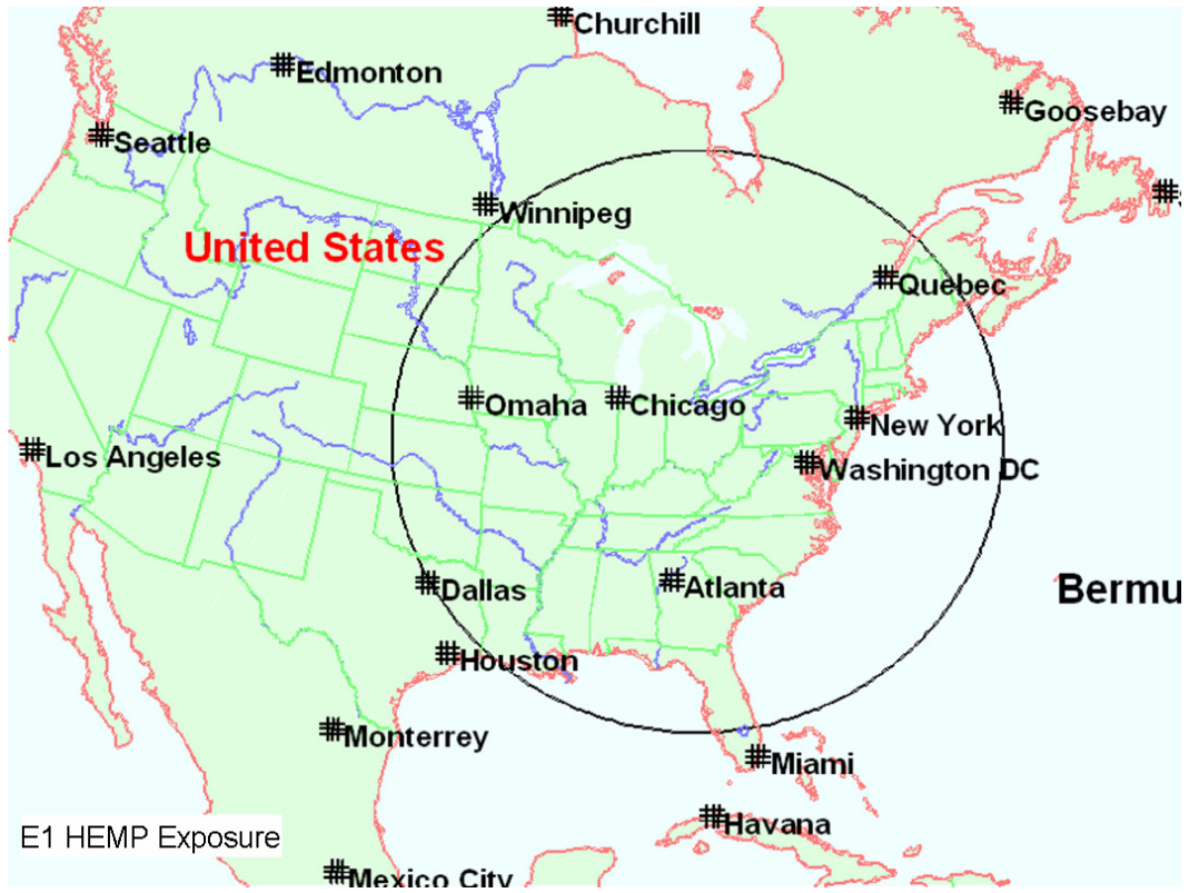
Figure 7-16. Exposure area for E1 HEMP burst at 170 km over Ohio.
