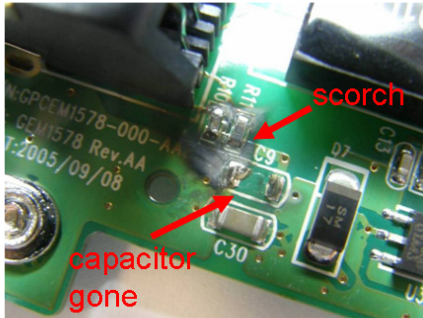
Figure 6-2. Capacitor damage from pulse testing. The capacitor (C9) is gone, and there are scorch marks (C30 shows an undamaged capacitor).
