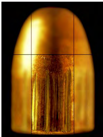
Figure 4-6. One of several land engraved areas (LEAS) on a fired bullet. Most common 9 mm bullets have 6 LEAS. Photo by Forensic Technology, Inc.
