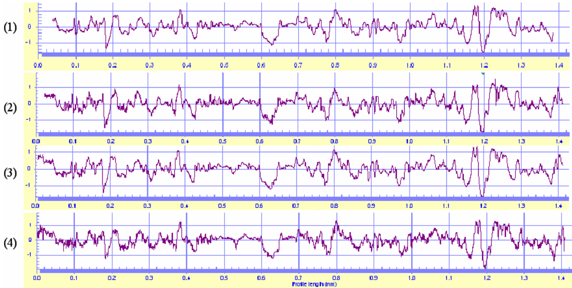
Figure 2-1. The profile of LEA 1 of a standard bullet measured by four techniques [24]. 1) stylus instrument; 2) interferometric microscope, CCF_{\max} = 92.1\% with respect to the stylus profile; 3) Nipkow-disk confocal microscope, CCF_{\max} = 98.9\% ; 4) laser scanning confocal microscope, CCF_{\max} = 95.3\% . The vertical unit is \mu\text{m} , the horizontal unit is mm.
