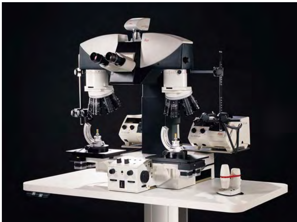
Figure 1-1. Photo of a forensic comparison microscope used to inspect pairs of objects and match images of similar objects. Inspection of the bases of a pair of cartridge casings is illustrated here (photo from Leitz* product literature).
