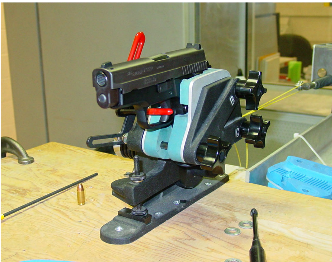
Figure 5-2 Photograph of one of the BIDE guns held in the fixture for remote test firing.
