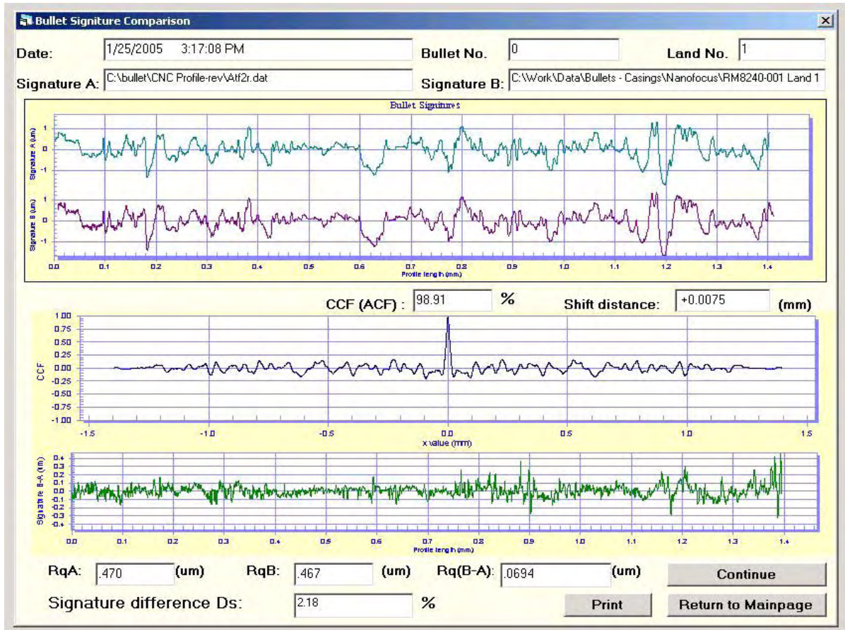
Figure 2-2. Computer screen showing a comparison of stylus (top) and Nipkow-disk (second) confocal profiles of LEA 1 of a standard bullet.
