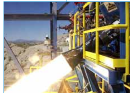
Microcosm's ablatively-cooled engine
