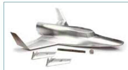
Lynx wind tunnel model with U.S. quarter (for scale)
