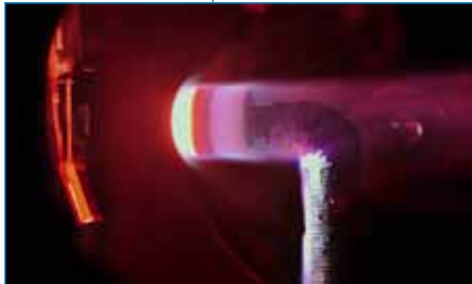
Testing of SpaceX's PICA heat shield material
