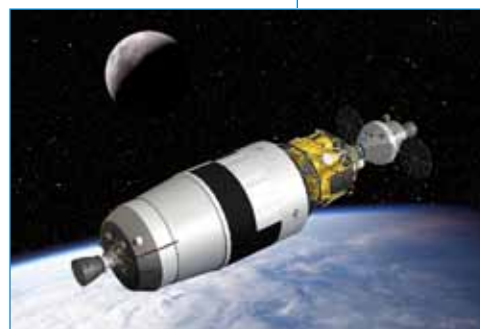
Artist rendition of the Ares V departure stage in orbit with the Orion capsule docked with the Altair lander
