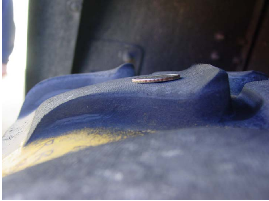
Figure 24. Left-Rear Tire After 60 Miles Without RWS
