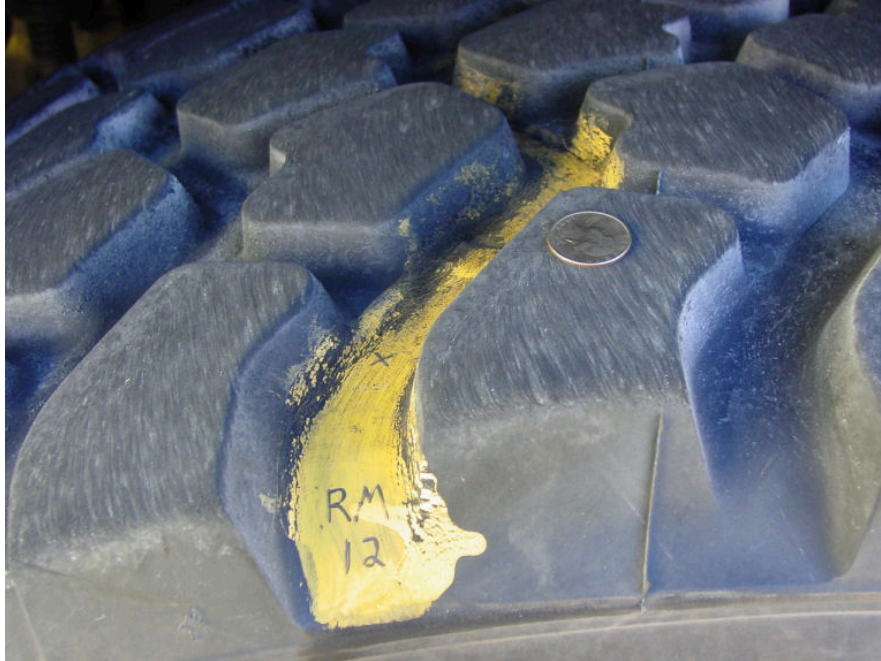
Figure 26. Right-Middle Tire After 60 Miles Without RWS
