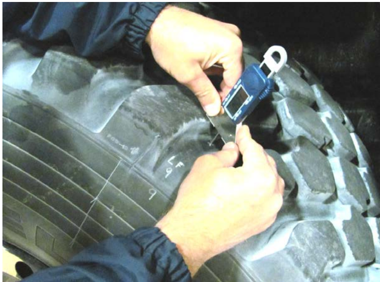
Figure 7. Measuring Tread Depth With Fowler X-Tread Gauge
