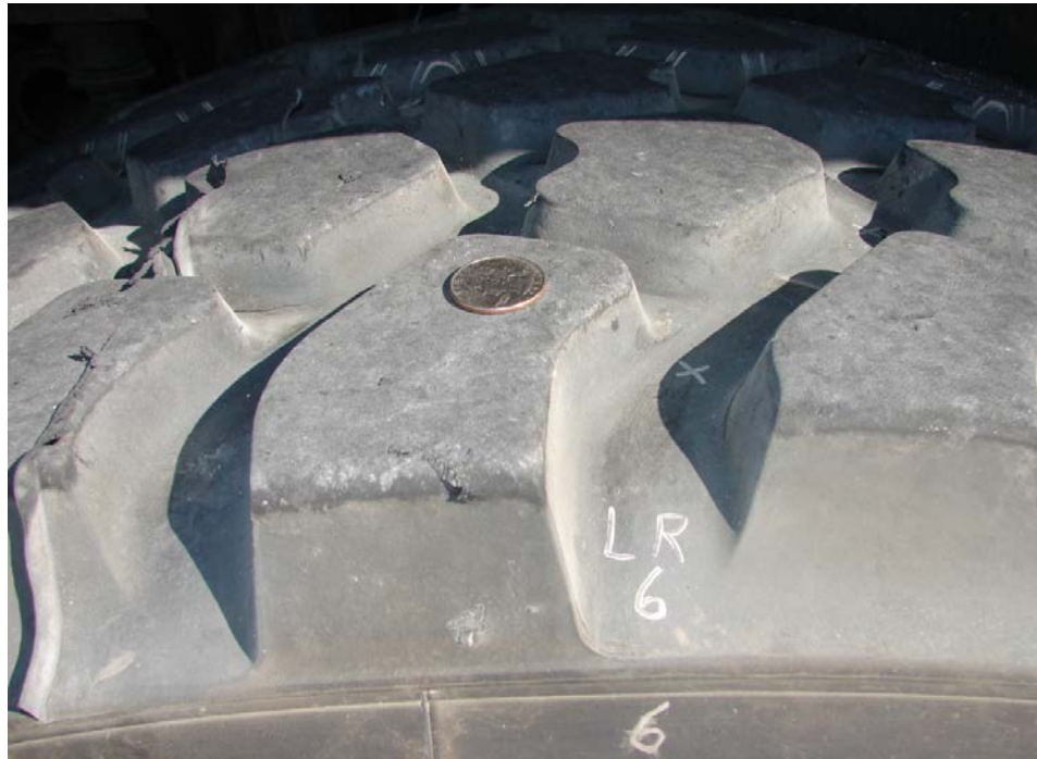
Figure 25. Left-Rear Tire After 60 Miles With RWS
