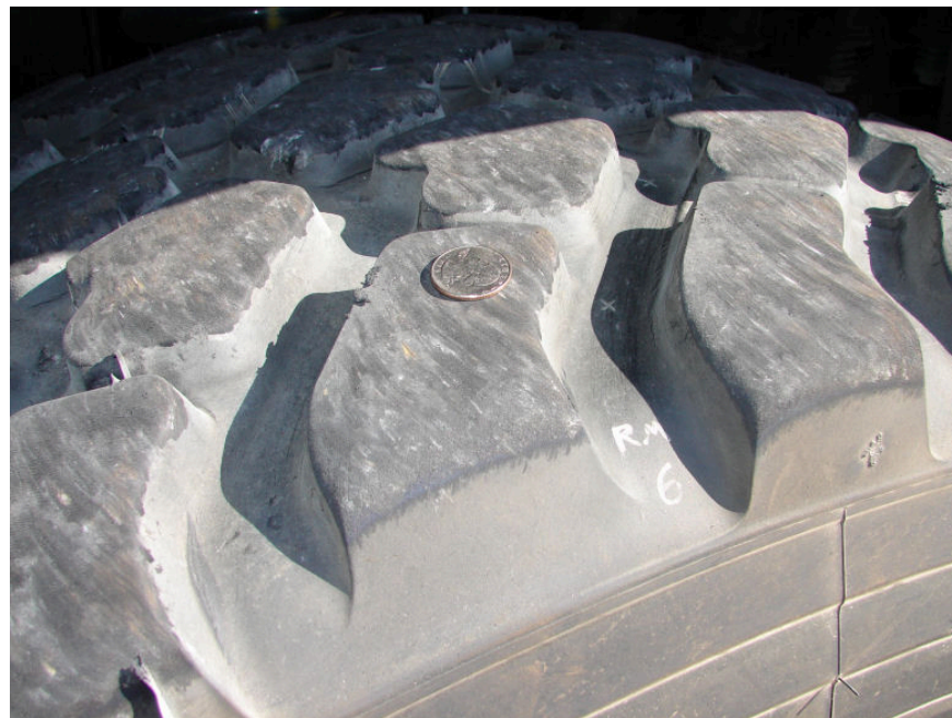
Figure 27. Right Middle Tire After 60 Miles With RWS
