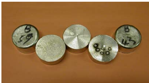
Semi-chill cast disks of SRM 1728 showing various stages in manufacturing and testing.
