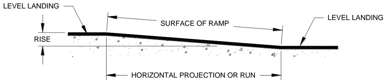
ELEVATION CHANGES GREATER THAN 0.50 in [13 mm] REQUIRE A SURFACE WITH A RECOMMENDED SLOPE OF 1:16 TO 1:20, BUT MUST NOT EXCEED THE FOLLOWING MAXIMUM SLOPES IN THE DIRECTION OF EXPECTED PASSENGER TRAFFIC:
