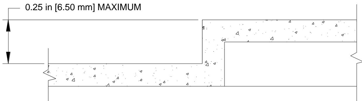
**Figure 4. Vertical Change in Level (cross section)**
