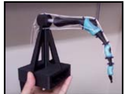
An anthropomorphic robotic finger with biomimetic finger joints. Courtesy of Professor Emanuel Todorov
