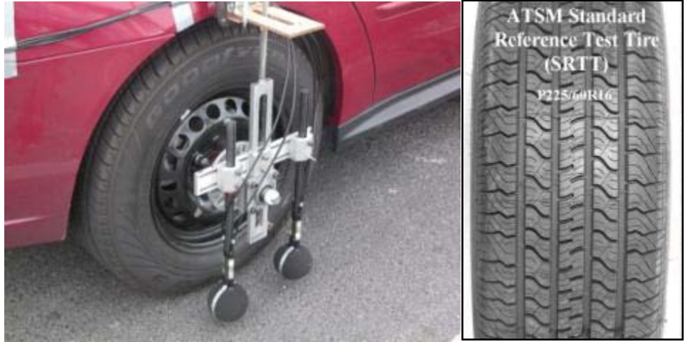
Figure 14. OBSI dual probe system and the SRTT.
