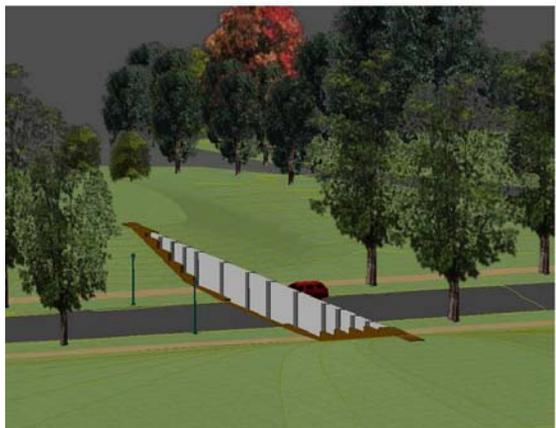
The improved levee will consist of a removable post-and-panel barrier system connected to permanent masonry walls and earthen berms designed to seamlessly blend with the setting of the National Mall.
