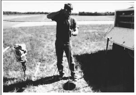
Figure 8.19. Starting the stainless steel rod with a hammer.
