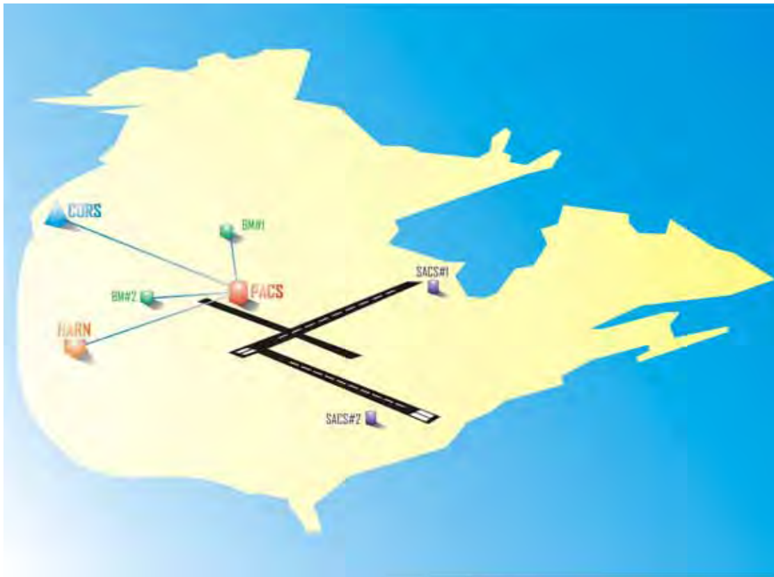
Figure 1.1. Illustrates the connection of the airport to other portions of a control network.
