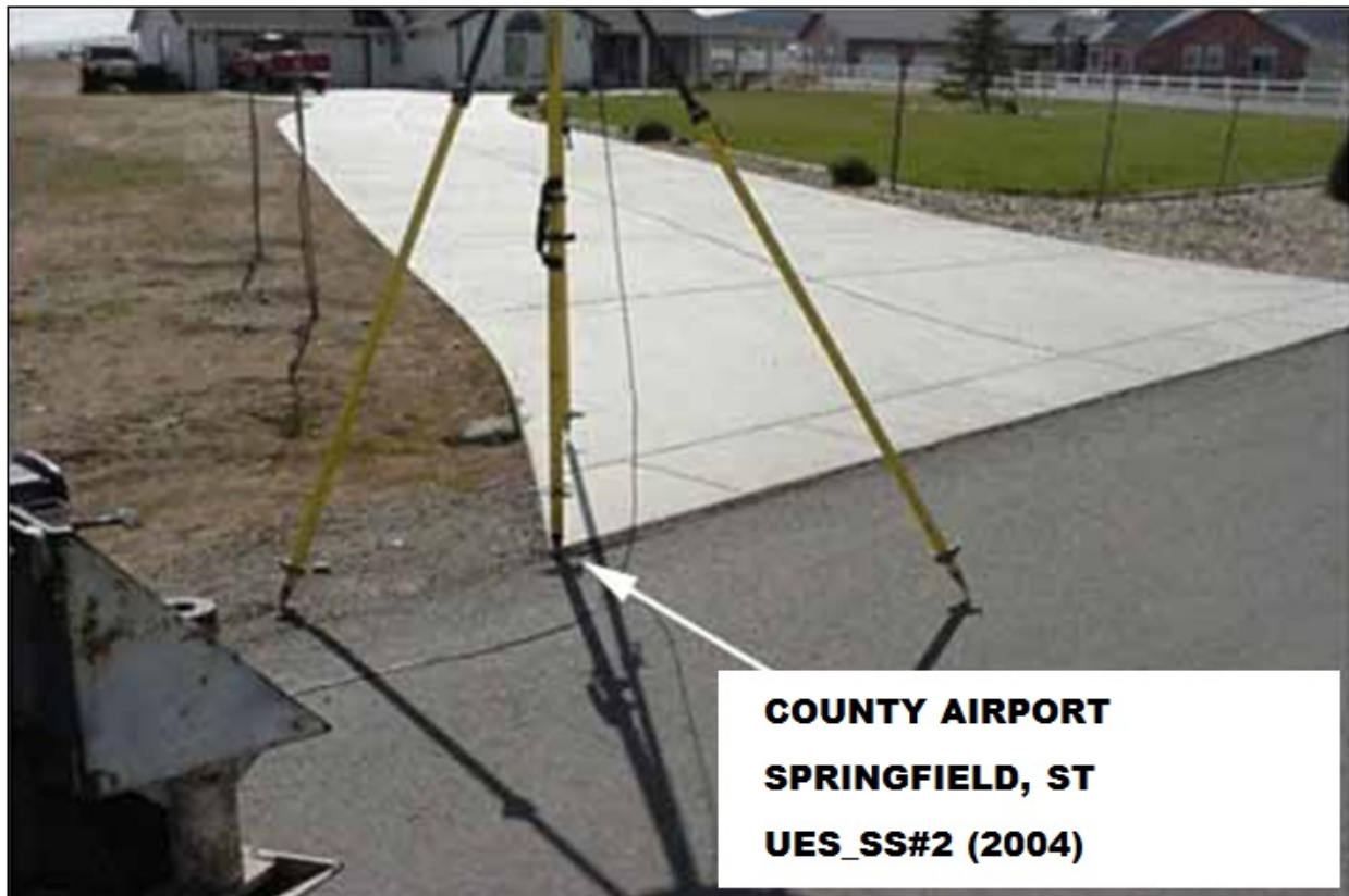
Figure 2-5 Sample Digital Photograph of Imagery Control Point with Antenna
