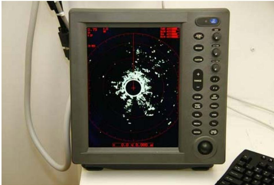
**Figure 2-2. A Radar Operational Console**
