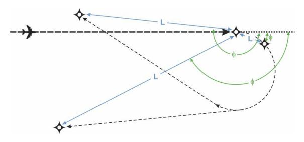
R=turn radius  $\phi$ =turn magnitude at segment initial fix
