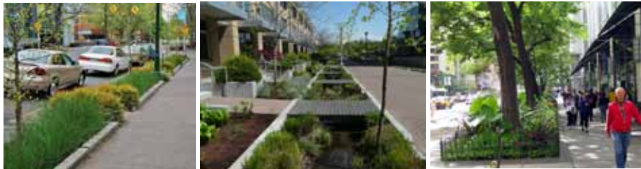
Green streets will be used to manage stormwater and improve urban ecology
