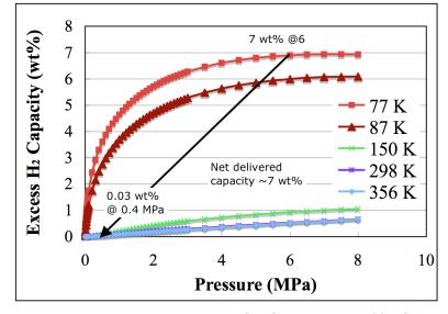
Dubinin-Astakhov Model Fit of MOF-177. >95% of stored  $H_2$  will be delivered at 4 bar or higher. Tank heats from 80 to 300 K during delivery.
