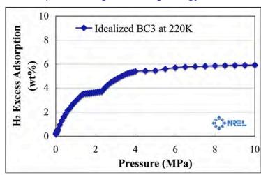
Idealized porous  $BC_3$  could deliver >5 wt%  $H_2$  (>50 g/L) at -50°C.
