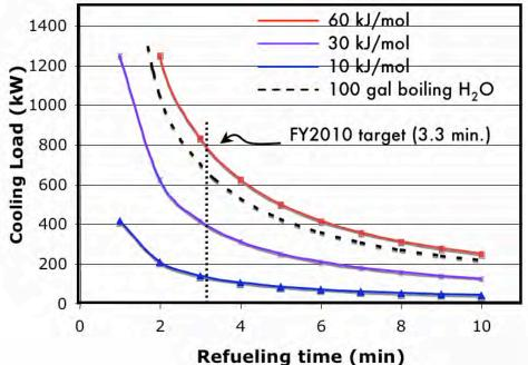
Cooling load for 5 kg of adsorbed H<sub>2</sub> for different binding
