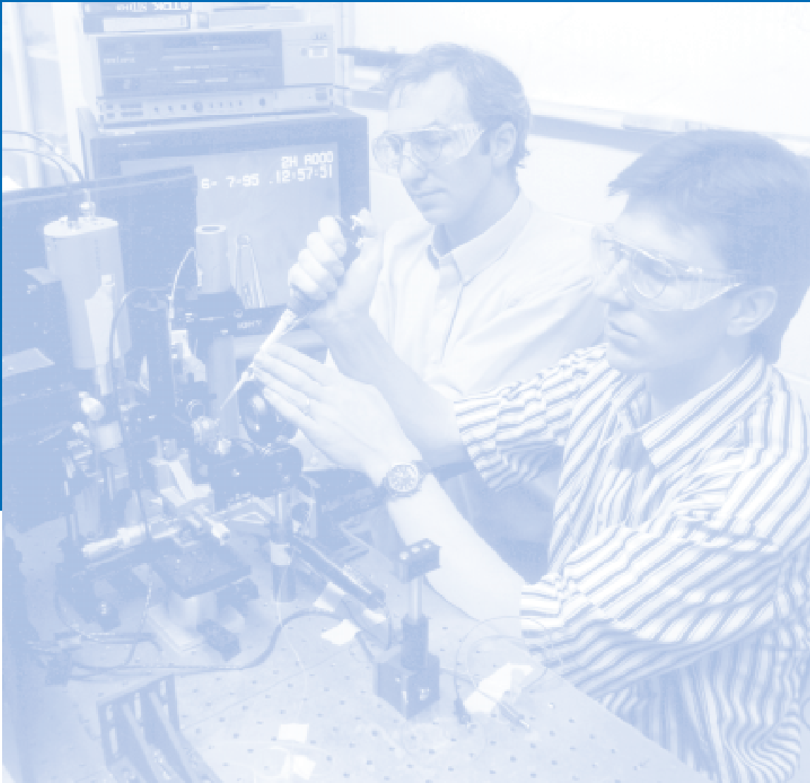
Los Alamos National Laboratory researchers Peter Goodwin and Rhett Affleck load a sample of fluorescently labeled DNA into an ultrasensitive flow cytometer used to detect single cleaved nucleotides. [Source: Lynn Clark, LANL]
