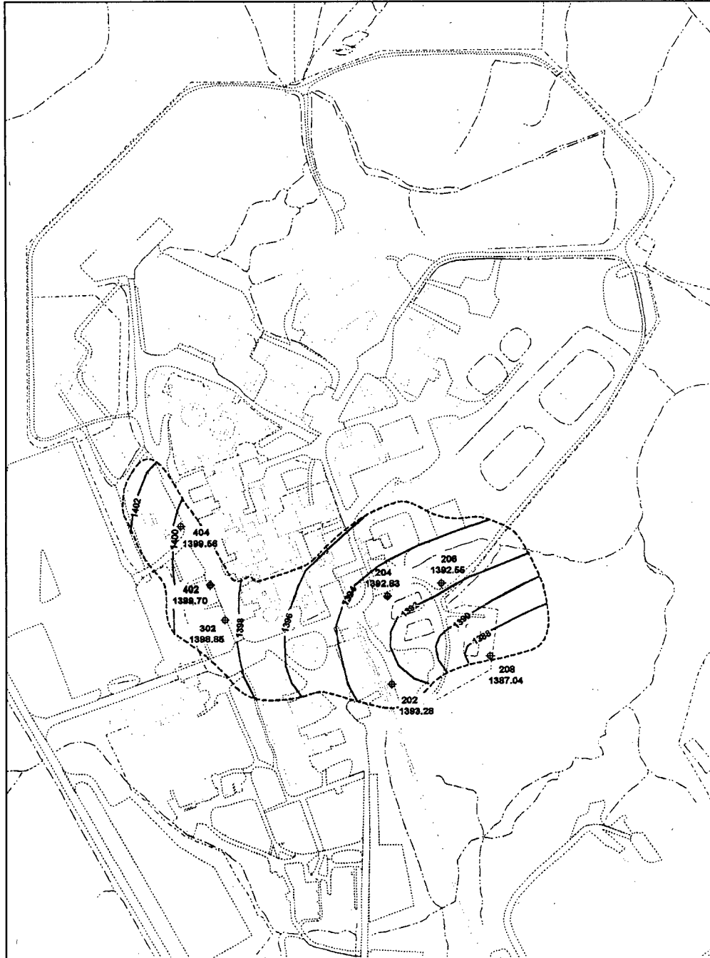
Figure 5C9-1. Pre-2007 Inferred Areal Extent of the Lavery Till Sand in the North Plateau
