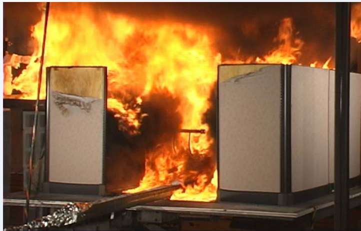
Single workstation burn tests for input to fire dynamics simulator
