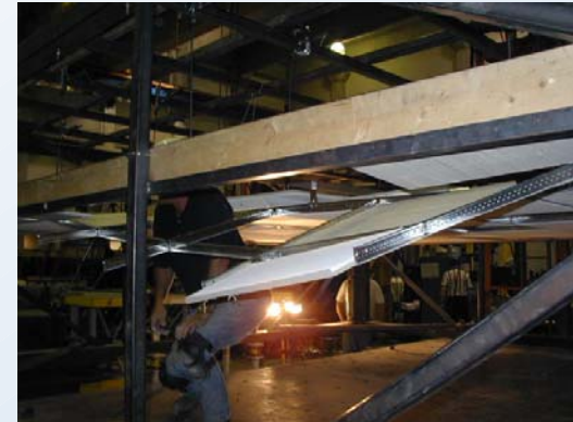
Assess the effect of impact on damage to ceiling tile systems
