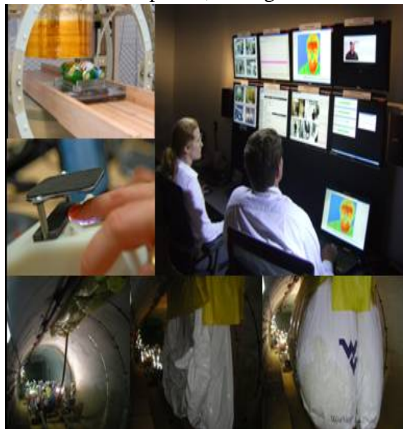
S&T's Innovation work includes liquid identification technologies for explosive detection at airports (top left), biometric identification and hostile intent detection (top right), contactless fingerprinting (middle left) and an inflatable tunnel plug to protect tunnels from fire and flooding (plug deploying – bottom row)
