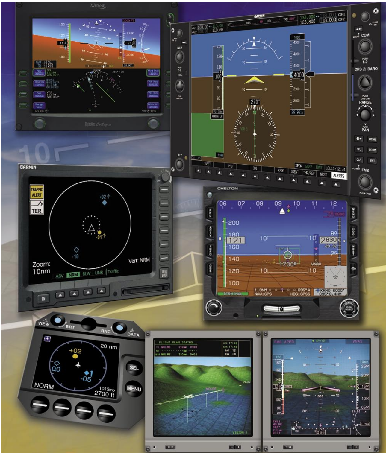
Figure 17-18. Electronic flight instrumentation comes in many systems and provides a myriad of information to the pilot.
